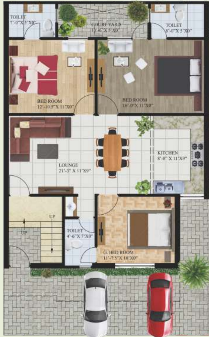
Ground Floor (Without Lift) 3BHK, 3 Toilet
